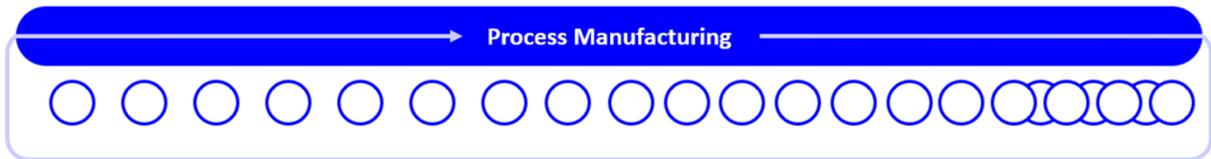
**Process manufacturing** does not have a distinct start or end, rather it is defined by its continuous combination of materials. Typical industries that use process manufacturing include chemical, food and beverage, pharmaceutical, oil and gas refining, cosmetics and textile dyeing.
