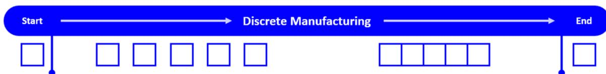
**Discrete manufacturing** refers to the production of individual parts or units that come together to create a final good through a series of specific and separate workflows. Typical industries include automotive, aerospace, consumer goods and electronics.
